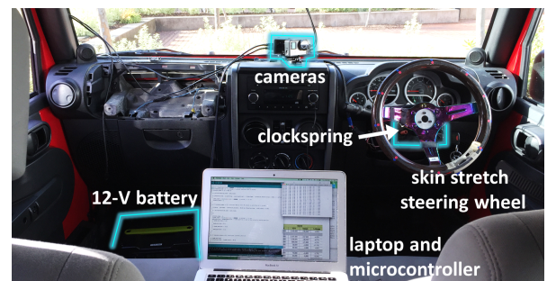
Fig. 3. The experimental setup in the vehicle consisted of the haptic steering wheel attached to the steering column, a clockspring to route the wiring, a laptop and microcontroller for the experimenter to control the haptic and audio cues and auditory N-back task, a camera system for data collection, and a 12V battery to power the haptic motor.
