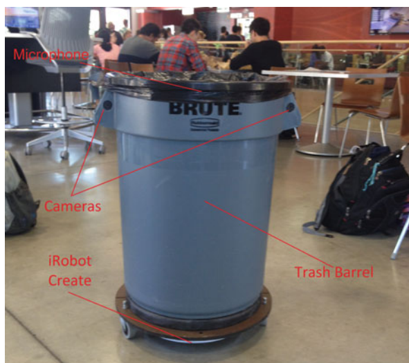
Fig. 8 A standard Rubbermaid Brute trash barrel is mounted atop an iRobot Create platform. A laptop computer, hidden within the trash barrel, handles video and control commands
