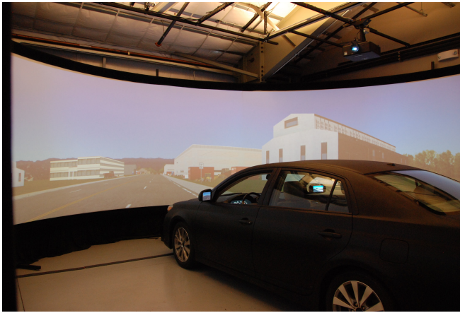
Fig. 2. Driving Simulator showing the 270° projection with side mirrors and in-simulator vehicle
