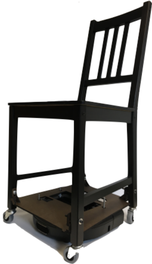
Fig. 1. Robotic furniture could be used in shared human spaces, re-organizing itself as needed. This paper explores the ability of a single ChairBot to communicate non-verbally with human bystanders.
