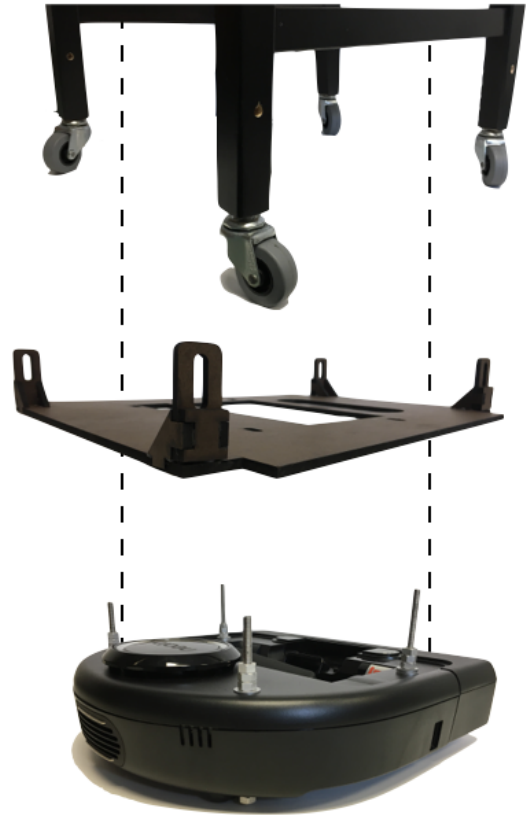
Fig. 3. Each ChairBot is comprised of a wooden IKEA chair with added castors, laser-cut chassis, and Neato Robotic Vacuum.
