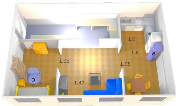
Fig. 2. A model of the visited smart-home. The numbers denote the width of door openings and other spaces, for example 1.51 m in the door opening to the bedroom and the width and depth of the kitchen is 1.8 m. The cylinder 'a' represents the Giraff and the office chair 'b' represents the wheelchair.
