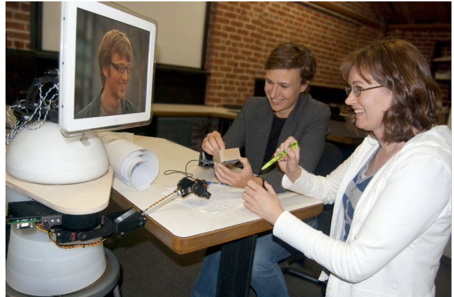
Figure 1: This telepresence robot prototype supports live audio and video of a remote collaborator on a remotely-controlled, movable screen. It has a robotic arm, allowing the collaborator to point and gesture expressively.
