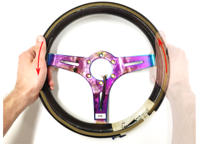
Fig. 1. Skin stretch steering wheel display: ring at front of the rim shown highlighted in yellow can rotate \pm 0.5 degrees, producing \pm 2.5 mm of skin stretch, and can be gripped anywhere. Integrated motor is visible at the 5 o'clock position
