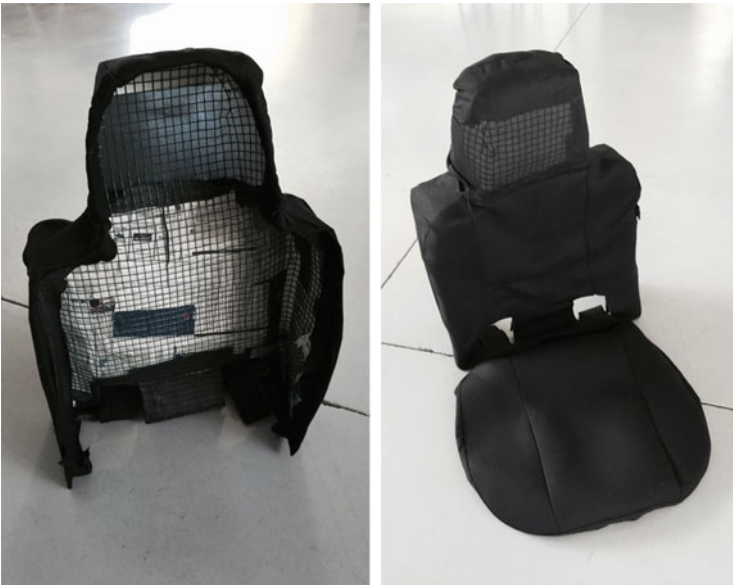
Fig. 8 The seat cover costume includes two arm outlets so that the concealed driver could steer the car using the bottom of the steering wheel
