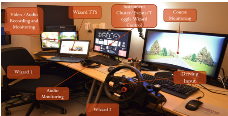
Fig. 2 The Wizard of Oz control station. Wizard 1 (the Interaction Wizard) interacts with the participant, while Wizard 2 (the Driving Wizard) initiates transfers of control and operates the vehicle during autonomous driving mode
