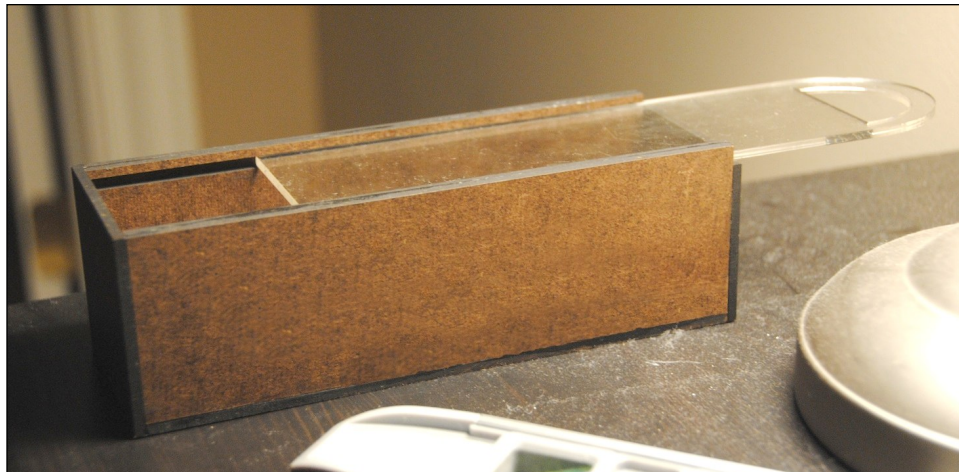
Figure 3: An example housing/box for homework 2, intended to hold small sketching and lab tools, and fabricated on a laser cutter from masonite and acrylic.
