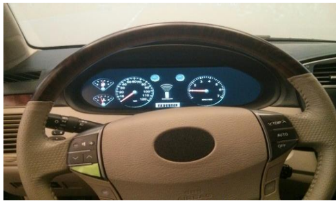
Figure 3. Steering wheel with mode switch button marked in green. The same button enables or disables the automated driving features, and the mode switch is only enabled in specific transition zones.
