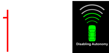
Figure 4. Automation system status indicator on instrument panel. The car icon lights up in green to indicate that the system is on, and turns to grey to when it is off. The arcs in front of the car show when the system is turning on or off, and descriptive text is provided below the vehicle icon.
